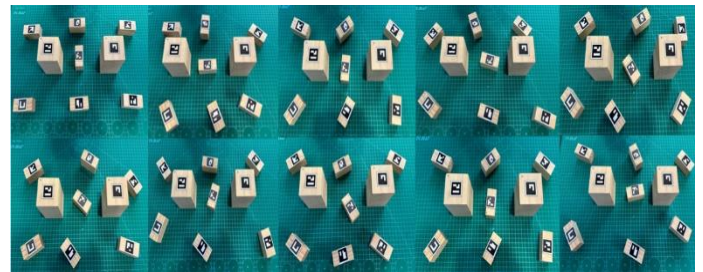
FIGURE 7: PICK AND PLACE EXPERIMENT (10 GROUPS IN TOTAL, 7 TARGET CUBES AND 2 OBSTACLE CUBES ARE PLACED RANDOMLY IN EACH GROUP.)
