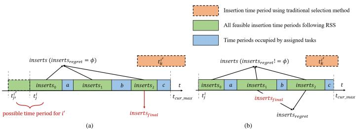
**FIGURE 4:** (A) A CASE WHEN THE IDENTIFIED TIME PERIODS FOR INSERTION OF TASK i ALLOW THE INSERTION OF NEXT TASK i'. (B) A CASE WHEN THE IDENTIFIED TIME PERIODS FOR INSERTION OF TASK i DO NOT ALLOW THE INSERTION OF NEXT TASK i'.
