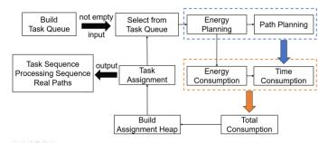
**FIGURE 2:** THE OVERALL FRAMEWORK OF INTEGRATED TASK AND PATH PLANNING APPROACH.
