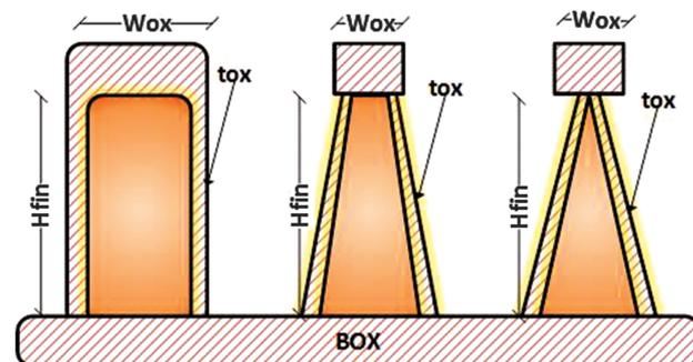
Fig. 8. Left side: A fin with a vertical slope which presents better short channel metrics.<sup>32</sup> Middle: A standard fin with some degree of inclination as the one used in the 22 nm Intel's node.<sup>26</sup> Right side: A fin with a triangular cross-sectional area that can help to reduce the leakage.<sup>33</sup>
