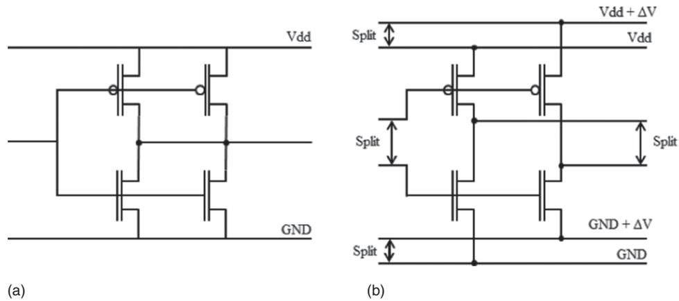
Fig. 11. (a) Static CMOS inverter with 2 fins per transistor and (b) Split-circuit inverter with split inputs, outputs, and supply rails.<sup>39</sup>
