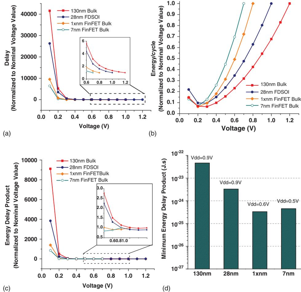
**Fig. 17.** (a) Delay versus  $V_{dd}$ ; (b) Energy/cycle versus  $V_{dd}$ ; (c) Energy Delay Product (EDP) versus  $V_{dd}$  and (d) Minimum EDP values across multiple technology nodes (simulated with the same NAND-based ring oscillator structure).
