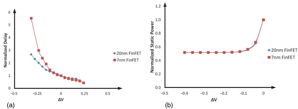
Fig. 12. Simulation results (using the predictive FinFET nodes<sup>40</sup>) with the Split-biasing circuit for a FFT butterfly module (a) Normalized delay from a change in inputs to a change in outputs; (b) Normalized static power in standby mode.<sup>39</sup>
