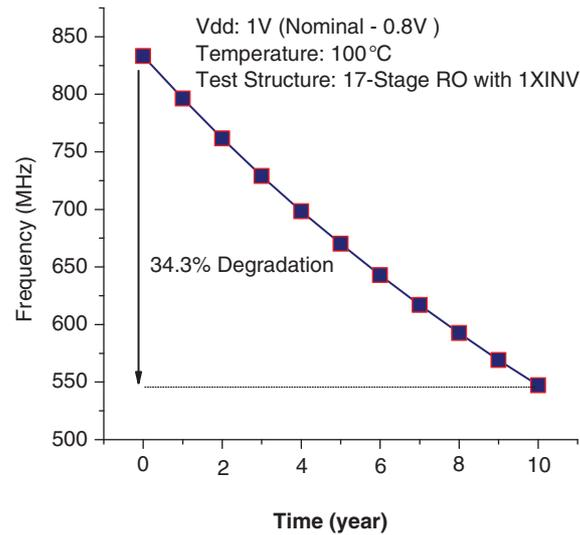
**Fig. 16.** Aging simulation with  $1 \times$  nm bulk FinFET with foundry-provided aging models (BTI+HCI).
