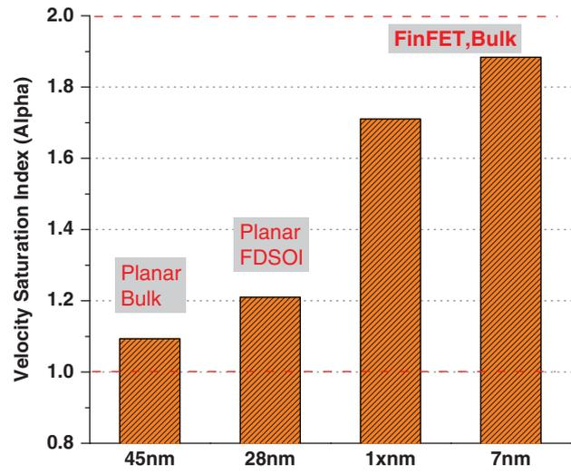
**Fig. 6.** Velocity saturation index ( $\alpha$ ) for different technologies.
