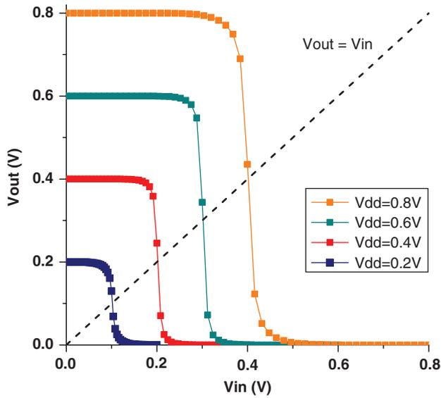
**Fig. 5.** VTC curves under different supply voltages for a 1xnm FinFET inverter (PMOS and NMOS are sized equally).
