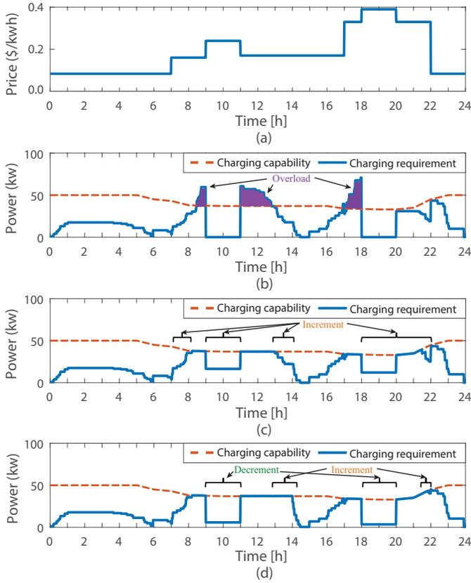
Fig. 5. (a) Electricity price profile. (b) Charging requirement of EVs by method-1. (c) Charging requirement of EVs by method-2. (d) Charging requirement of EVs by method-3.
