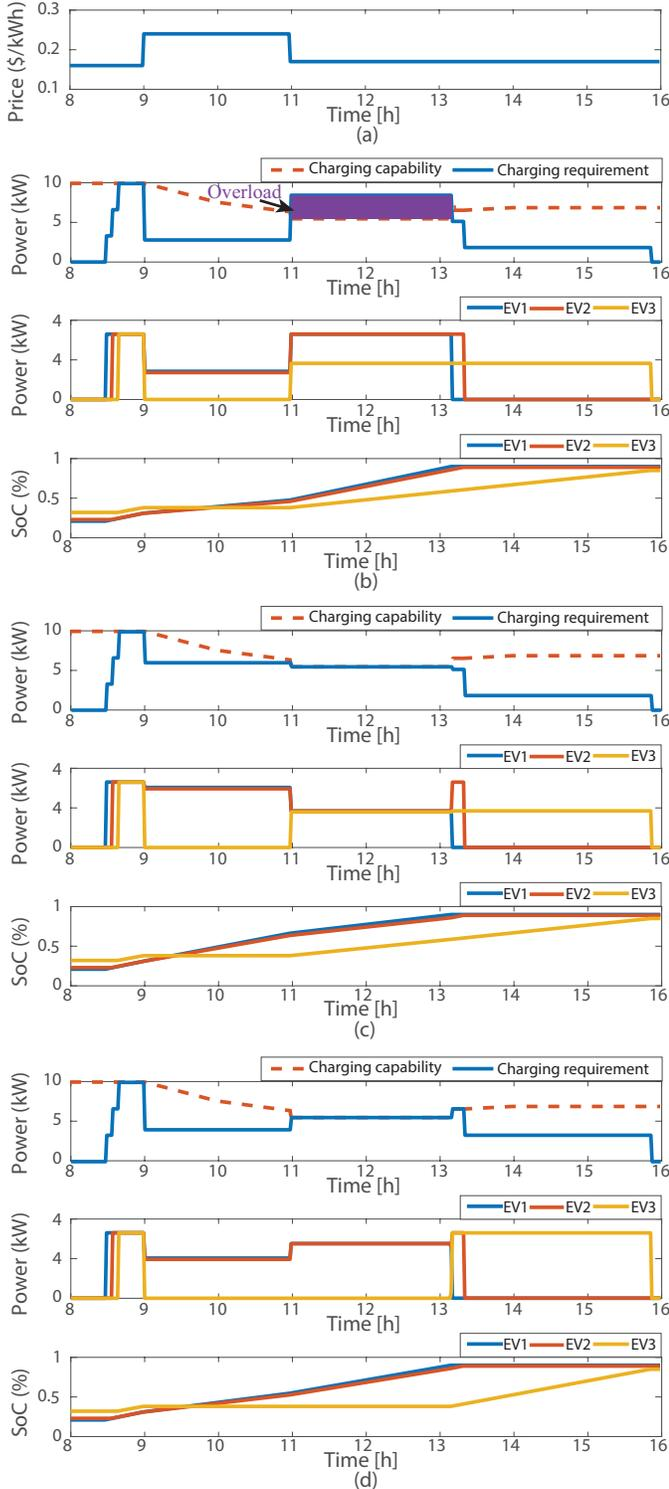
Fig. 4. (a) Electricity price profile. Charging capability, charging requirement, and EVs' responses of power and SoC in (b) Method-1. (c) Method-2. (d) Method-3.
