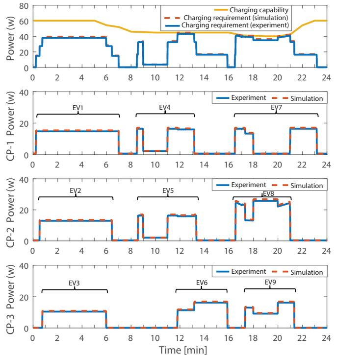
Fig. 8. Experimental versus simulation results (CP: charging pole).
