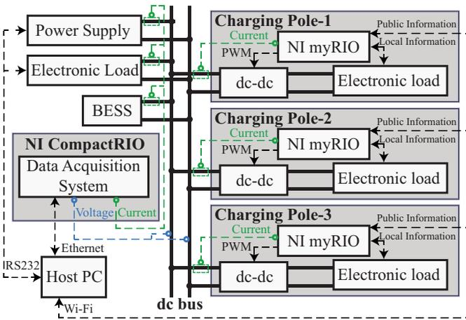
Fig. 7. Functional block diagram of the testbed.
