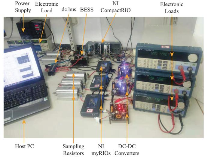
Fig. 6. Downscaled testbed.
