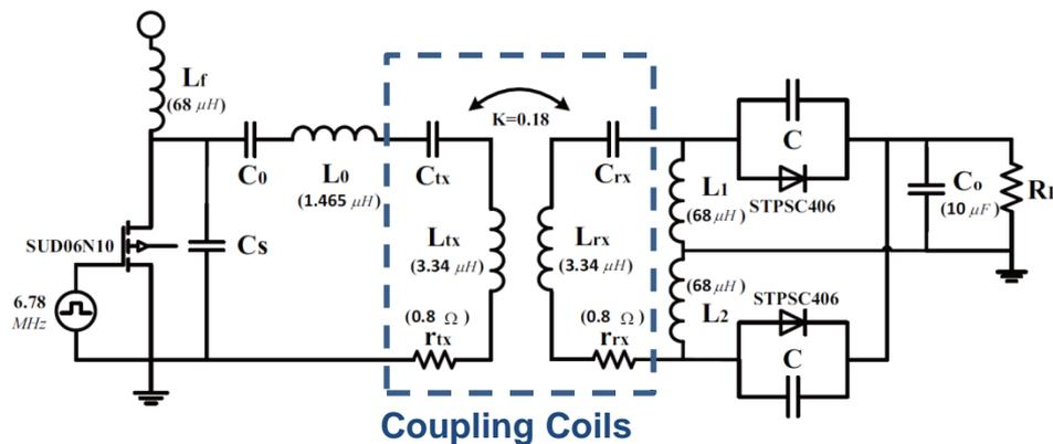
Due to the series-series compensation, the input and output currents of the coupling coils are sinusoidal. Thus the THDs of their input/output voltages are criteria to verify the improvement on EMI.
