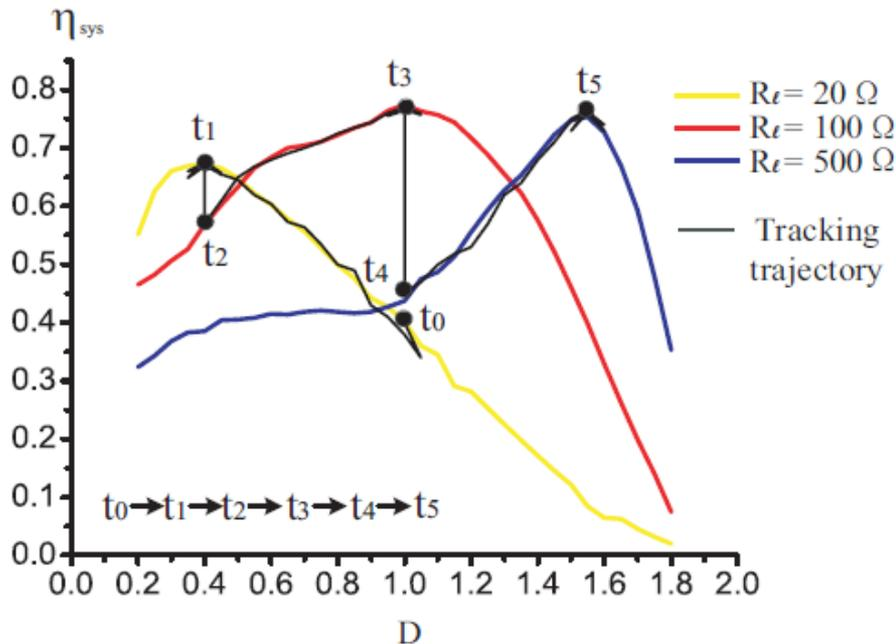
Fig. 1 Tracking of optimal load resistances with a varying  $R_L$ .
