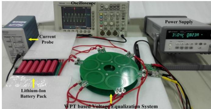
Multi-receiver MHz WPT-based cell equalization
