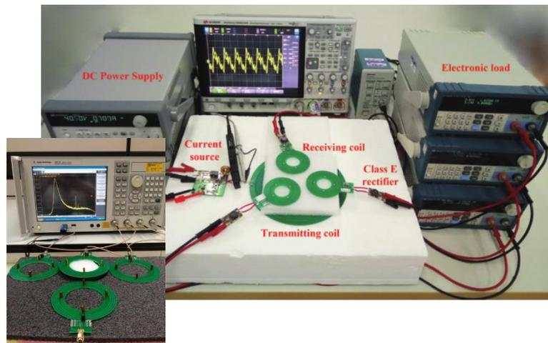
Compensation and autonomous power distribution in multi-receiver WPT systems
