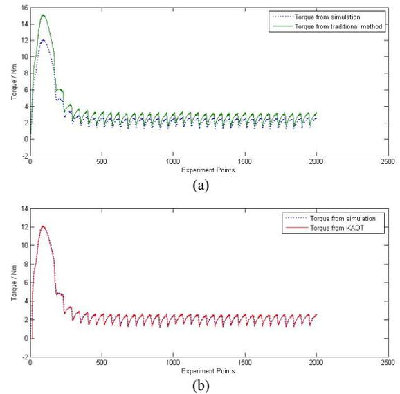
Fig. 7 Torque Calculation Result at High Temperature with (a) Traditional Method and (b) KAOT
