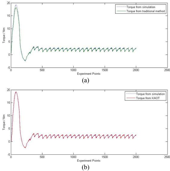
Fig. 6 Torque Calculation Result at Low Temperature with (a) Traditional Method and (b) KAOT
