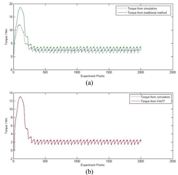
Fig. 8 Torque Calculation Result when aging with (a) Traditional Method and (b) KAOT
