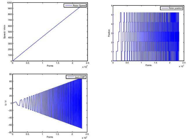
Fig. 2 Rotor Speed, Position and Back EMF
