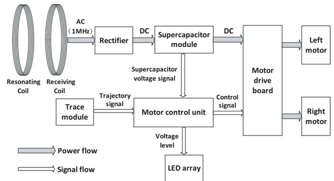
Figure 6. The configuration of the supercapacitor model vehicle
