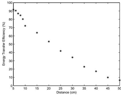
Figure 11. Resonant coil distance versus energy transfer efficiency
