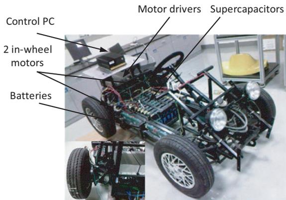
Figure 14. Experimental one-seat electric vehicle
