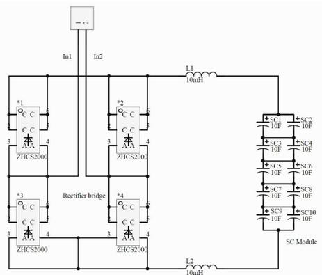
(b) Schematic circuit diagram of rectifier and supercapacitors
