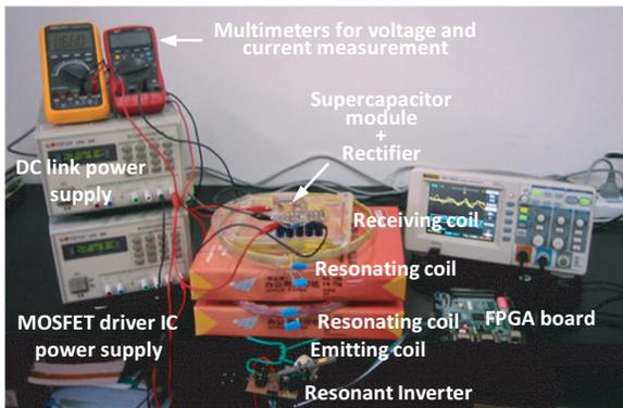
Figure 8. The experimental setup
