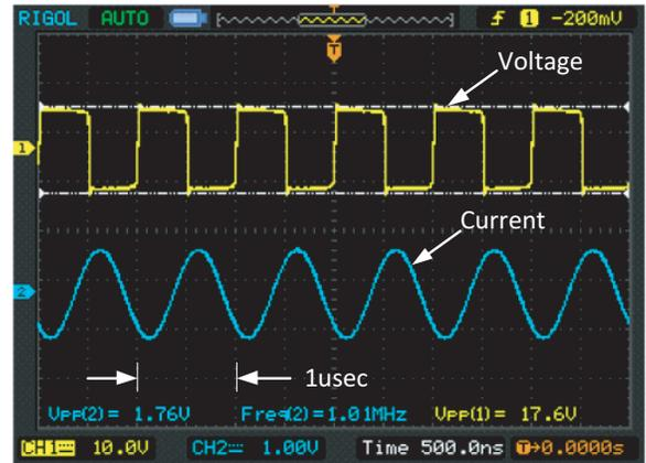
Figure 9. The voltage and current waves in the emitting coil
