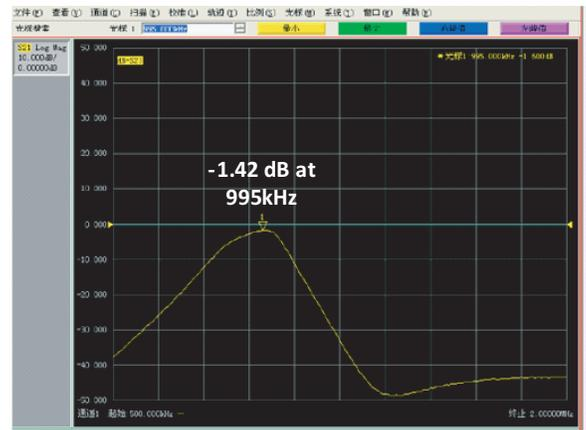
Figure 10. Transmission characterization of coils by network analyzer
