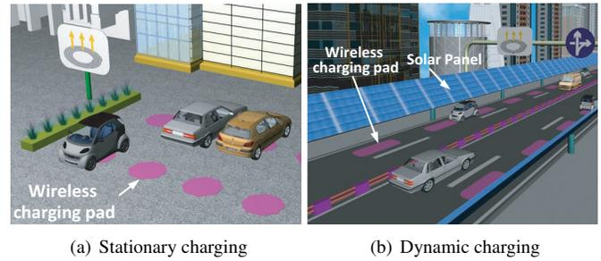
Figure 1. Future electric vehicle wireless charging systems
