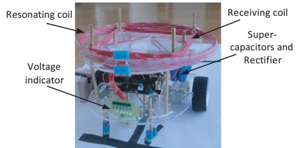
Figure 4. The wirelessly charged supercapacitor model vehicle
