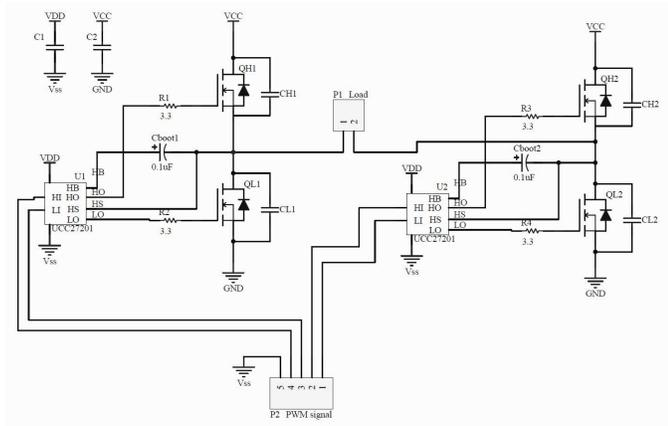
(a) Schematic circuit diagram
