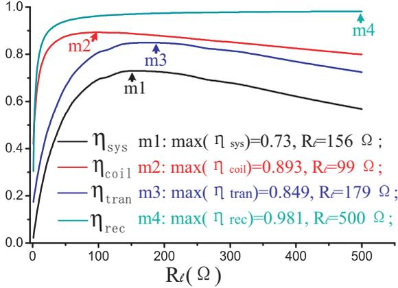
Figure 6: Efficiency curve under various  $R_l$  when  $k = 0.12$ .
