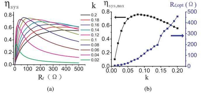
Figure 7: System efficiency and optimal load for the coupling system with the rectifier. (a) Efficiency curve under various  $k$  and  $R_l$ . (b) Maximum system efficiency and optimal  $R_l$  under various  $k$ .
