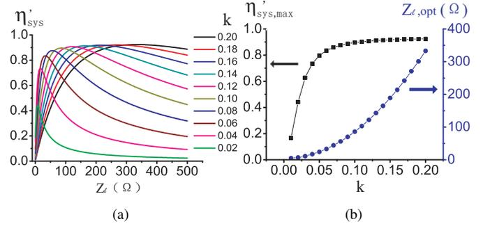
Figure 4: Maximum efficiency and optimal  $Z_l$  under various  $k$  for the coupling-only system.
