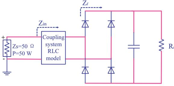
Figure 5: System configuration with a rectifier.
