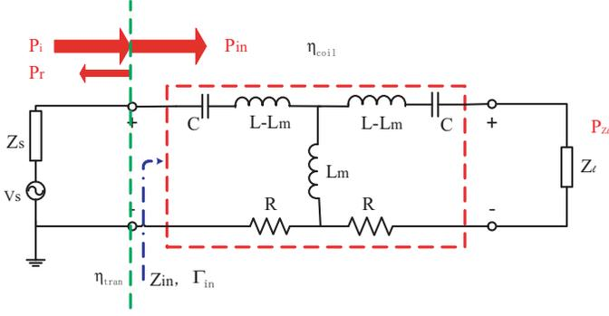
Figure 2: Equivalent circuit model of a WPT system.
