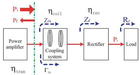
Figure 1: System configuration.
