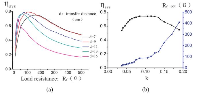
Figure 11: System efficiency and optimal load in experiments. (a) Efficiency curve under various  $R_l$  and transfer distance. (b) Maximum system efficiency and optimal load under various  $k$ .
