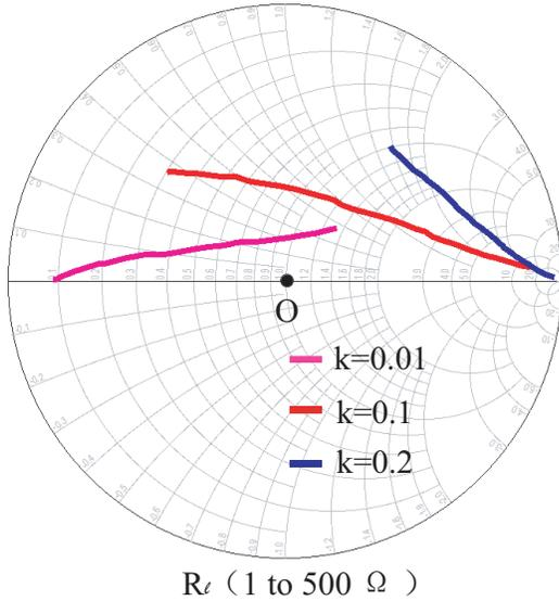
Figure 9:  $Z_{in}$  under different  $R_l$  when  $k = 0.01, 0.1$  or  $0.2$ .
