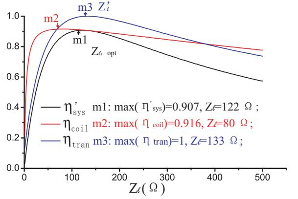
Figure 3: Efficiencies comparison by sweeping  $Z_l$  when  $k = 0.12$ .
