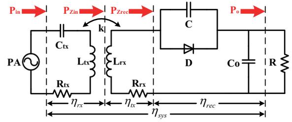
Fig. 3. The proposed compact Class E rectifier.
