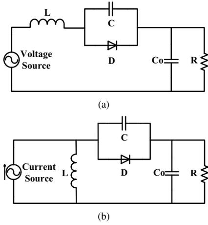
Fig. 1. Typical circuit model. (a) Voltage driven Class E rectifier. (b) Current driven Class E rectifier.
