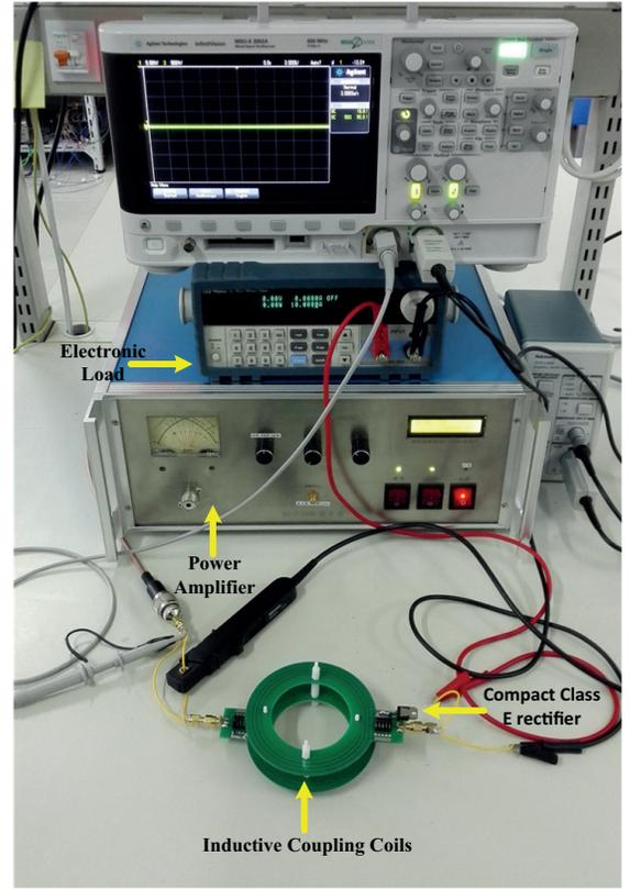
Fig. 9. The experiment setup.
