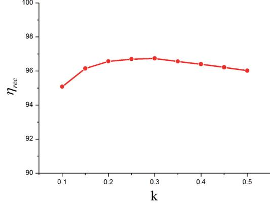
Fig. 6. The rectifier efficiency for different  $k$  when  $R = 32 \Omega$ .
