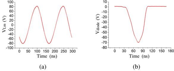
Fig. 5. Simulation results. (a) The voltage across  $L_m$ . (b) The voltage across diode.
