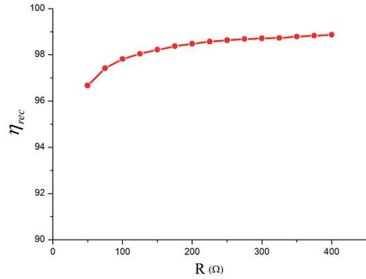
Fig. 7. The rectifier efficiency for different  $R$  when  $k = 0.3$ .
