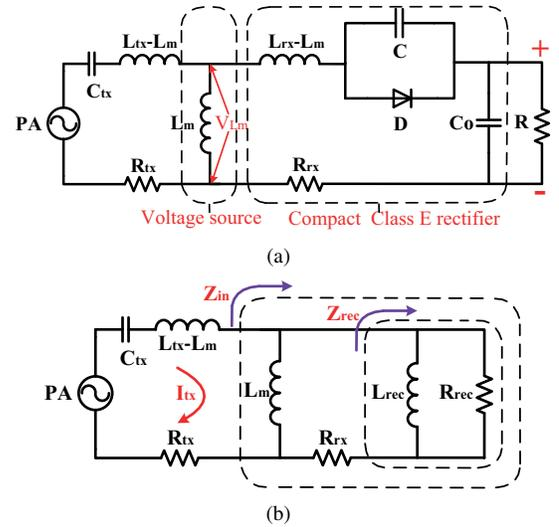
Fig. 4. Equivalent circuit model. (a) The proposed rectifier. (b) The circuit model based on [11].
