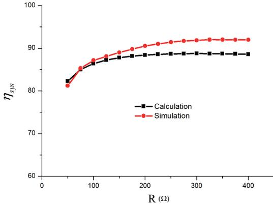
Fig. 8. The system efficiency of calculation and simulation for different  $R$ .
