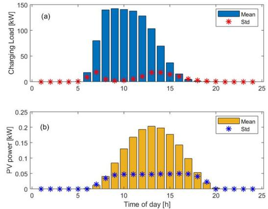
Fig. 4. Gaussian distribution parameter at each time instant: (a) Charging demand, (b) PV power.
