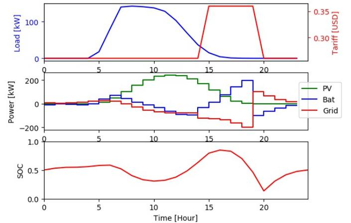
Fig. 5. Power flow in the charging station.
