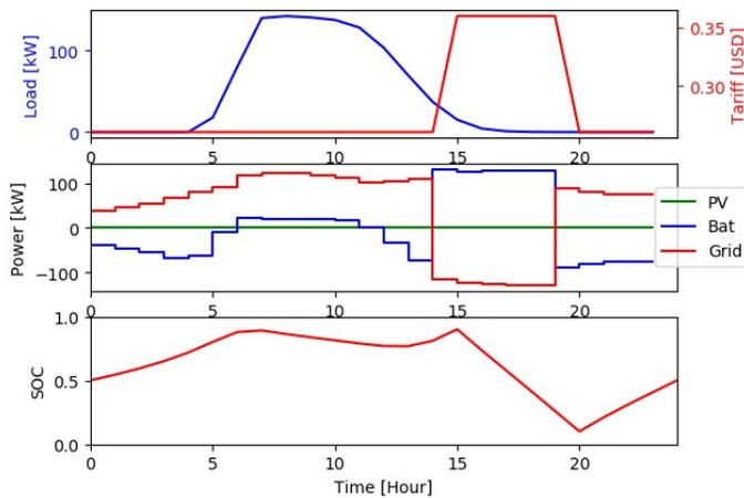
Fig. 6. Power flow in the charging station without PV system.
