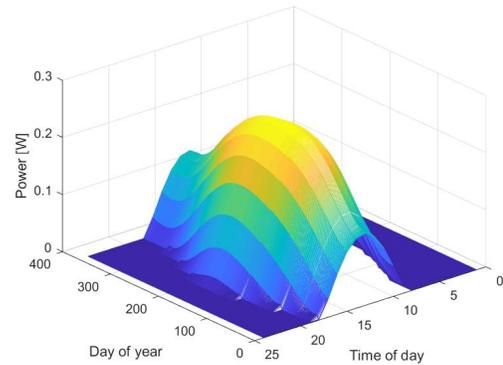
Fig. 3. One year power generation profile of a PV unit.
